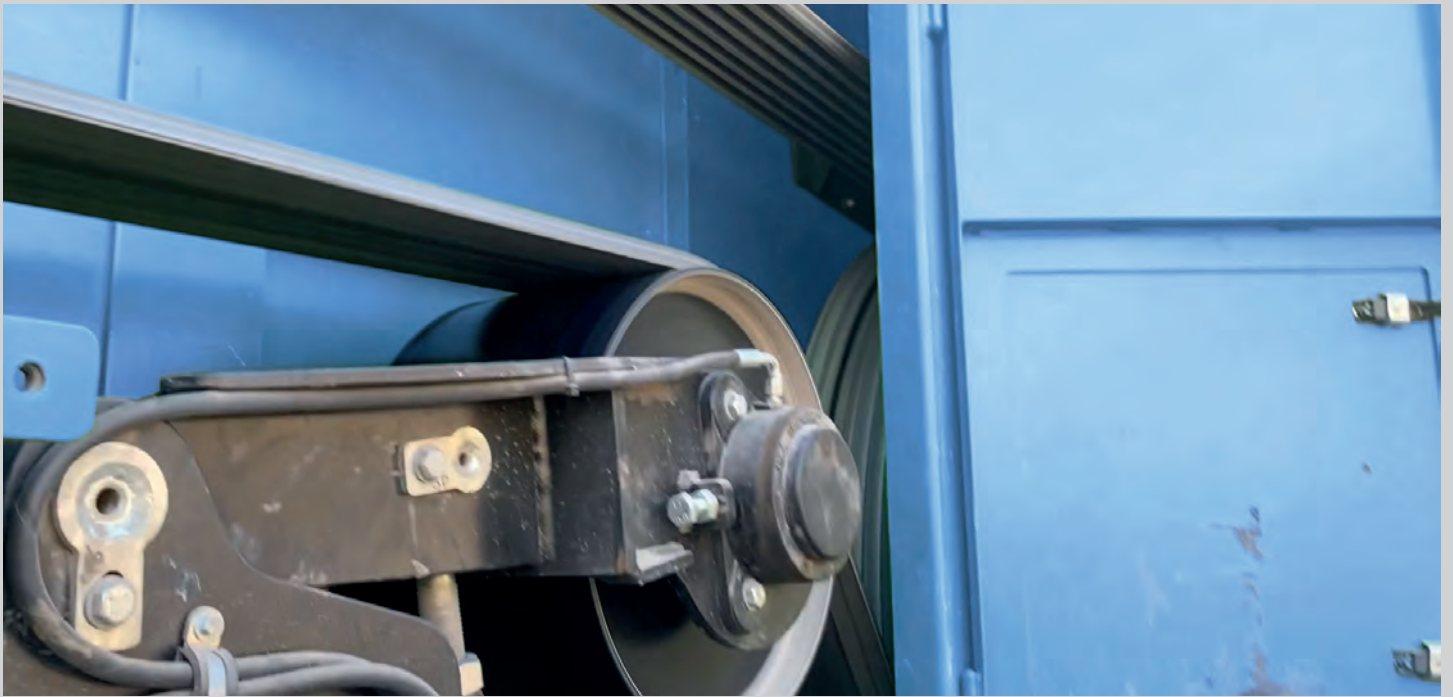
Power Guard® R-SPC10600 Multibelt running in a stone crusher drive at 42 m/sec.
