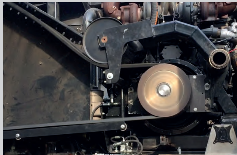
Power Guard® Multibelt in a wood shredder drive.
